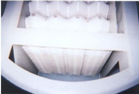
Inlet end showing plate pack, flow window and sealing plates
